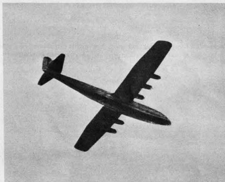
Six engines on 150-ft. wing give BV-222 speed of 240 m.p.h. Vast bulk, drooping nose, single fin and rudder are outstanding features.
